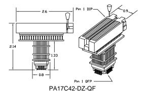
Note: DIP Pin 1 is in the lower right corner. Microchip packaged the QFP device with a180 degree rotation from the DIP & PLCC packages.
